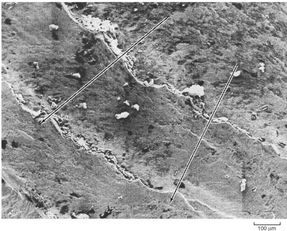
Fig. 6.15 Scanning electron microscope views of the fracture surfaces of the gear fragment. 100×
